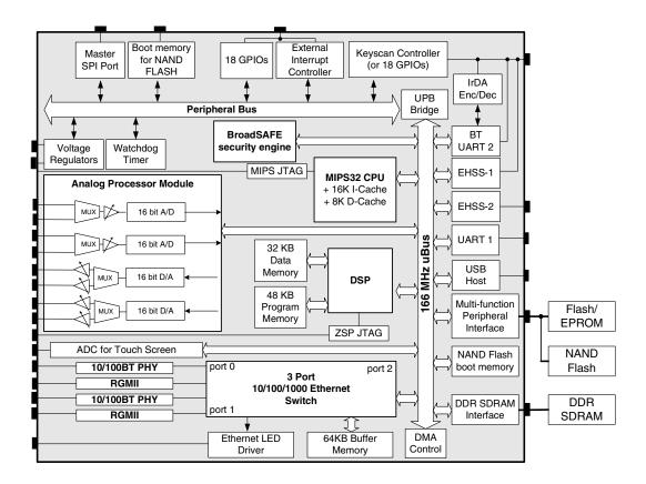
The Broadcom BCM1103 IP phone chip enables manufacturers to build IP phones with integrated Gigabit Ethernet switching, improved voice quality, hardware security and advanced graphics-driven applications.
