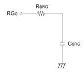
Reset gate clock equivalent circuit
