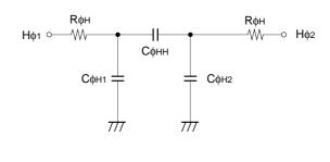
Vertical transfer clock equivalent circuit
