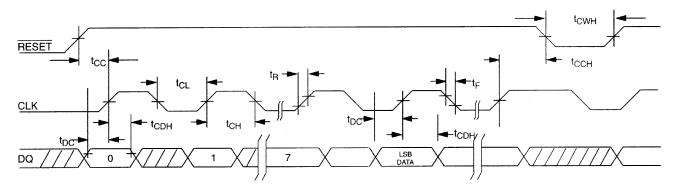
NOTE:  $t_{CL}$ ,  $t_{CH}$ ,  $t_R$ , and  $t_F$  apply to both read and write data transfer.
