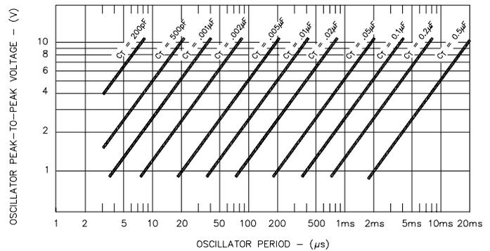
FIGURE 1 - SG1731 OSCILLATOR PERIOD VS.  $V_{osc}$  AND  $C_T$
