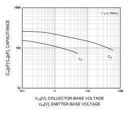
Figure 3. Output and Input Capacitance vs. Reverse Voltage
