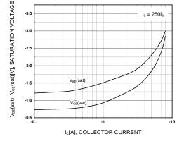
Figure 2. Base-Emitter Saturation Voltage Collector-Emitter Saturation Voltage
