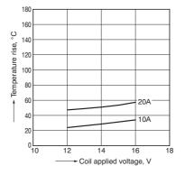
2. Ambient temperature and operating voltage range Sample: ACTG1H4
