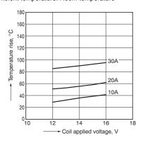
1.-(2) Coil temperature rise (at 110°C 230°F) Sample: ACTG1H4, 3pcs. Contact carrying current: 10A, 20A
