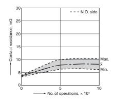
5.-(2) Electrical life test (Lamp load) Sample: ACTG1H4, 6pcs. Load: inrush: 84A/steady: 12A 14V DC Operating frequency: ON 1s, OFF 14s Ambient temperature: Room temperature Circuit:
