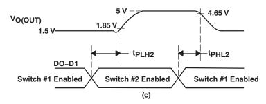
Figure 1. Propagation Delays and Transition Timing Waveforms
