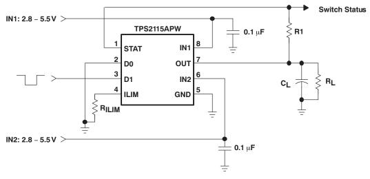
Figure 15. Manually Switching Power Sources
