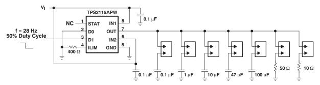
Output Switchover Voltage Droop Test Circuit Figure 5.
