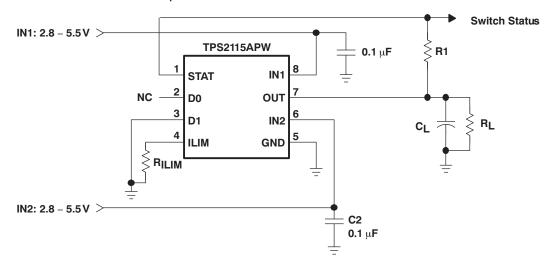
Figure 14. Auto-Selecting for a Dual Power Supply Application
