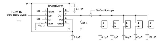
Output Capacitor Inrush Current Test Circuit Figure 7.
