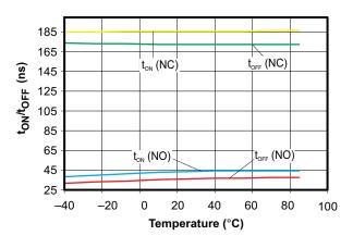
Figure 8.  $t_{ON}/t_{OFF}$  vs Temperature
