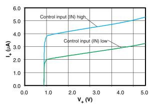
Figure 5.  $I_+$  vs  $V_+$  ( $T_A = 25$ °C)
