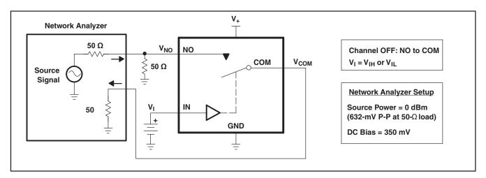
Figure 21. OFF Isolation (O<sub>ISO</sub>)
