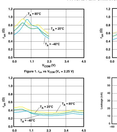
V<sub>COM</sub> (V) Figure 3.  $r_{on}$  vs  $V_{COM}$  ( $V_{+} = 4.5 \text{ V}$ )
