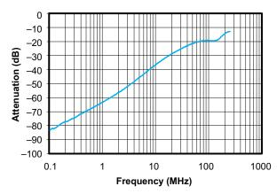
Figure 12. Crosstalk vs Frequency
