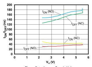
Figure 7. t<sub>ON</sub>/t<sub>OFF</sub> vs Supply Voltage
