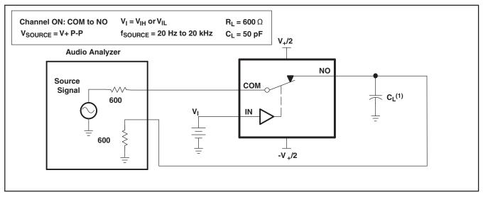
A. C<sub>L</sub> includes probe and jig capacitance.
