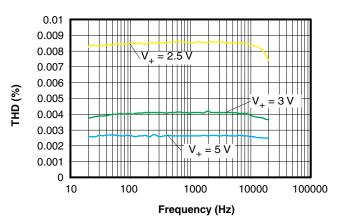
Figure 13. Total Harmonic Distortion (THD) vs Frequency
