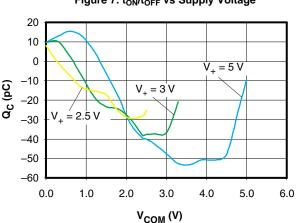
Figure 9. Charge Injection (Q<sub>C</sub>) vs V<sub>COM</sub>
