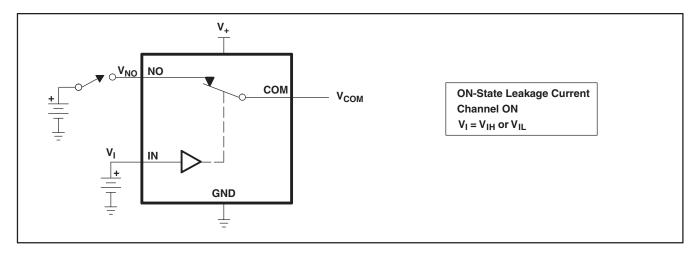
Figure 16. ON-State Leakage Current (I<sub>COM(ON)</sub>, I<sub>NC(ON)</sub>)
