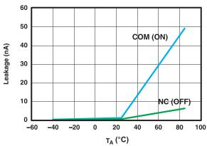
Figure 4. Leakage Current vs Temperature ( $V_{+} = 5 \text{ V}$ )
